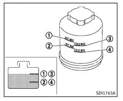
Check the fluid level in the reservoir.
