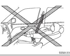
senger sits well back and straight up in the seat. If the seatback is reclined, the risk of sliding under the lap belt and being injured is increased.
