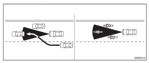
The detection zone of the ICC sensor is limited. A vehicle ahead must be in the detection zone for the vehicle-to-vehicle distance detection mode to maintain the selected distance from the vehicle ahead.
