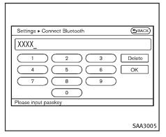
4. Choose a PIN code to use with the compatible Bluetooth<sup>®</sup> audio device using the number input screen. The PIN code will need to be entered into the Bluetooth<sup>®</sup> audio device after step 5. Select the "OK" key.
