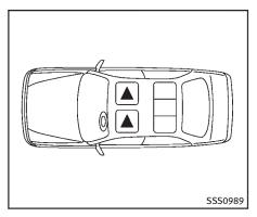
The illustration shows the seating positions equipped with head restraints. The head restraints of the front seats are adjustable.
