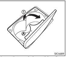
Automatic transmission models — Front To open the cup holder, push the lid (1). The flap (A) will be folded down when inserting a large container.
