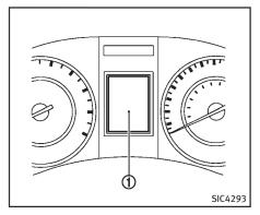
The dot matrix liquid crystal display ① is located between the tachometer and the speedometer, and it displays the automatic transmission position indicator (if so equipped), the Intelligent Cruise Control (ICC) system (if so equipped) information, the Intelligent Key operation information and other warnings and information.
