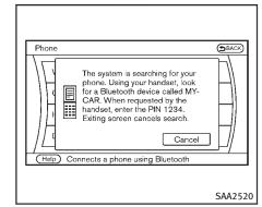
2. When a PIN code appears on the screen, operate the compatible Bluetooth<sup>®</sup> cellular phone to enter the PIN code.
