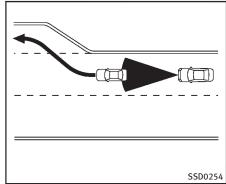
When driving on some roads, such as winding, hilly, curved, narrow roads, or roads which are under construction, the ICC sensor may detect vehicles in a different lane, or may temporarily not detect a vehicle traveling ahead. This may cause the ICC system to decelerate or accelerate the vehicle.
