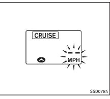
**To set cruising speed,** accelerate your vehicle to the desired speed, push the COAST/SET switch and release it. (Vehicle ahead detection indicator, set distance indicator and set vehicle speed indicator come on.) Take your foot off the accelerator pedal. Your vehicle will maintain the set speed.
