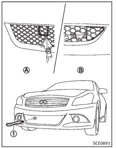
2. Securely install the vehicle recovery hook ① stored with jacking tools as illustrated. Attach the tow strap to the recovery hook.
