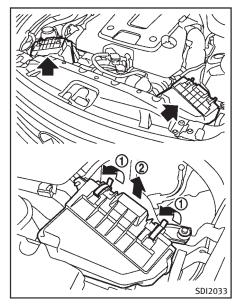
Remove the retainers (1) as illustrated and pull out the filter element (2).
