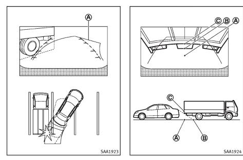
Backing up near a projecting object The predictive course lines (A) do not touch the object in the display. However, the vehicle may hit the object if it projects over the actual backing up course.
