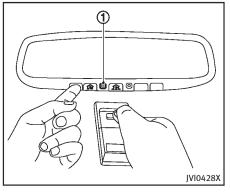
Using both hands, simultaneously press and hold the desired HomeLink<sup>®</sup> button and handheld transmitter button. DO NOT release until the HomeLink<sup>®</sup> indicator light ① flashes slowly and then rapidly. When the indicator light flashes rapidly, both buttons may be released. (The rapid flashing indicates successful programming.)
